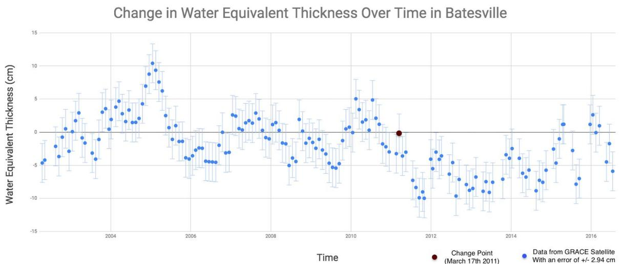
**Figure 3:** Change in water equivalent thickness over time for the Batesville region. The red dot indicates the change point on March 17th 2011.
