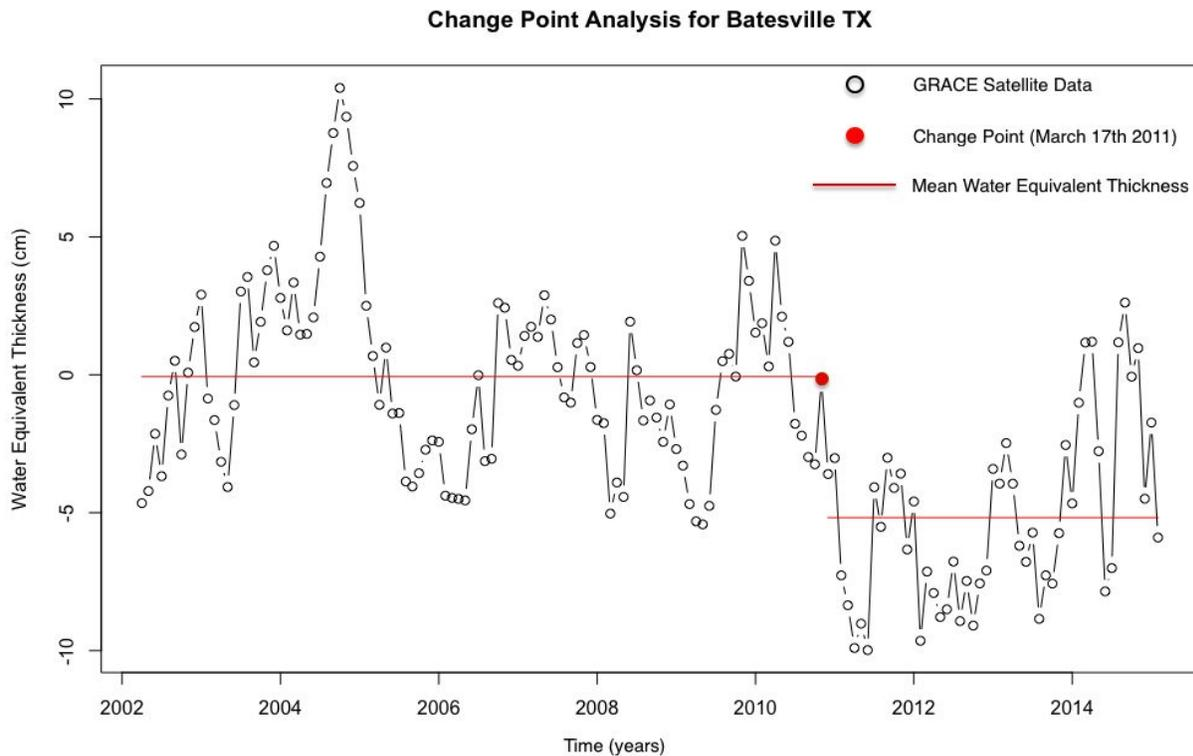
**Figure 4:** Change in water equivalent thickness over time. Here we can see the mean water equivalent changed from -0.07cm to -5.18 cm after the change point.
